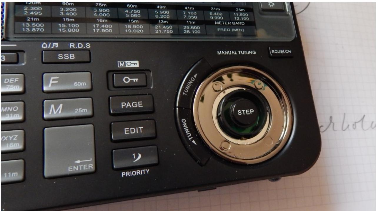
Good experience in unsoldering and the use of a vacuum pump to remove the incremental switch from the printed circuit board is essential. Some mechanical parts are made of plastic and overheating must be avoided. The opening of the rotating mechanism through very careful unbending of 4 metal stripes was more work as expected. But everything went well.
